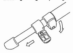
Open the Leg Lock Lever for extending/folding of tripod legs.
