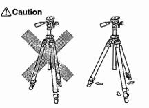
Prevent accidental equipment fall, or tripod tipping over, by making sure all levers, knobs, and handles on the tripod are securely tightened, and that all three legs are opened all the wav.
