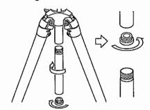
Remove the center column Base Stopper and then, remove the lower part of the center col-
