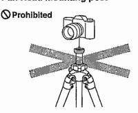
5 kgs (11 lbs), such as long lenses, may not balance well due to its weight distribution. In such case, please use a larger tripod.
